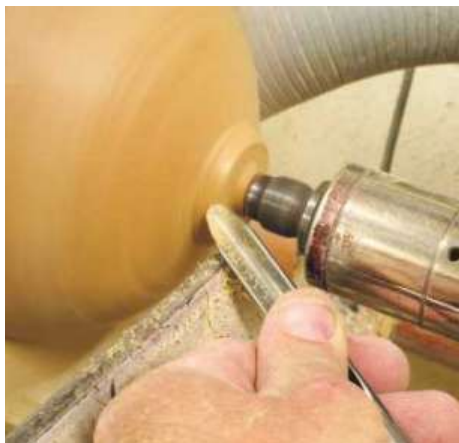
▲ Pic.34 Mount the bowl between centres with only enough pressure to drive the piece. Make light cuts using a small tool to clean up and shape the foot of the bowl
